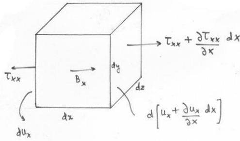
The increment of work done by the stresses  $\tau_{xx}$  on face 1 and by  $\tau_{xx} + \frac{\partial \tau_{xx}}{\partial x} dx$  on face 2 during infinitesimal displacement  $du_x$  at face 1 and  $d\left[u_x + \frac{\partial u_x}{\partial x} dx\right]$  at face 2 is:
