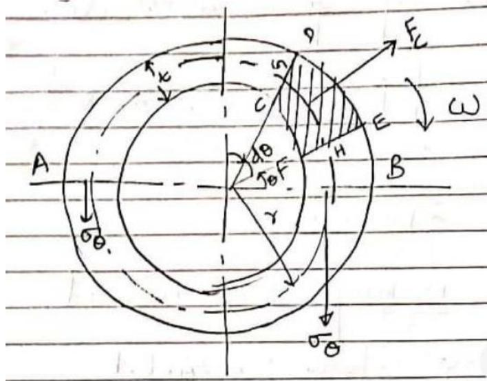
Consider a thin ring rotating about its centre of gravity at “o” as shown.
