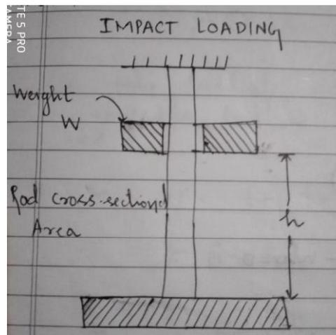
A prismatic linear elastic of crosssectional area \$A\$ and length \$L\$ (negligible mass) is hanging freely ,when a rigid weight \$W\$ is allowed to fall freely from a height on the rod as shown in fig. end of the rod contains flanges (wt. = 0kg ). Assuming no energy loss, calculate the longitudinal extension of rod due to impact.
