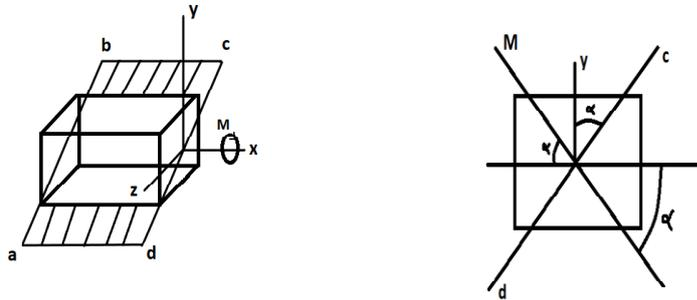
Assuming elastic behaviour of the material super-position of stresses caused by  $m_y$  and  $m_z$  is the solution of the problem
