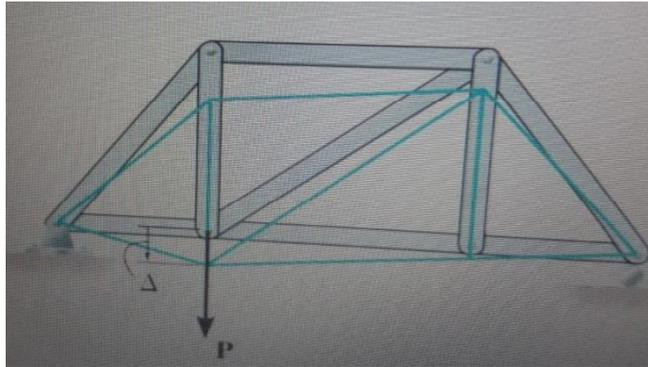
$$\frac{1}{2} P \Delta = \sum \frac{N^2 L}{2AE} \quad \left[ \frac{N^2 L}{2AE} = \text{strain energy by stress distribution} \right]$$
