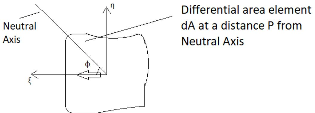
$\eta, \xi$  are the principal axis of area moment of inertia through the centroid.
