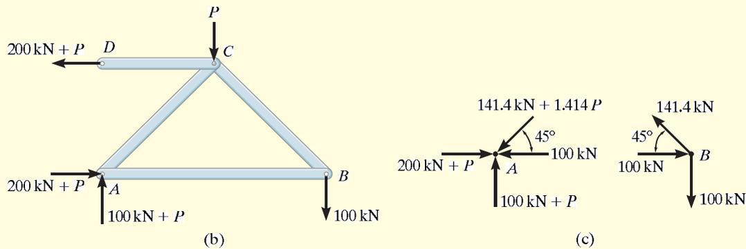
**Internal Forces  $N$ .** The reactions at the truss supports  $A$  and  $D$  are calculated and the results are shown in Fig. . Using the method of joints, the  $N$  forces in each member are determined. For convenience, these results along with their partial derivatives  $\partial N/\partial P$  are listed in tabular form. Note that since  $\mathbf{P}$  does not actually exist as a real load on the truss, we require  $P = 0$ .
