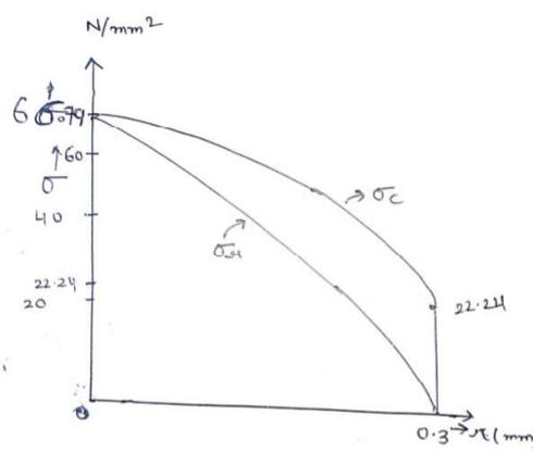
**Ex:** Hollow cylinder 20mm external radius and 100mm internal radius is rotating at 300rpm , density( $\rho$ ) = 7800 kg/m<sup>3</sup> and poisson's ratio ( $\mu$ ) = 0.3 ; Calculate maximum stress in cylinder . Plot variation of radial and hoop stresses?
