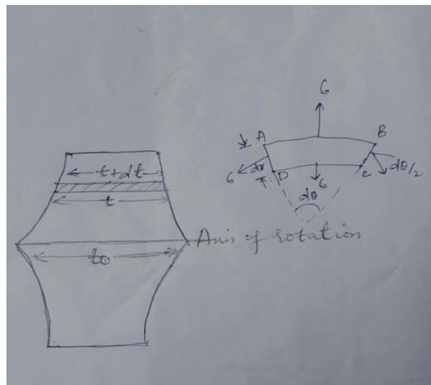
$\sigma$  = uniform stress in radial and circumferential direction.
